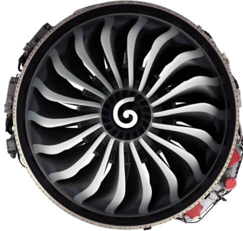
Typical CFM56 Engine Inlet Dome Spiral
